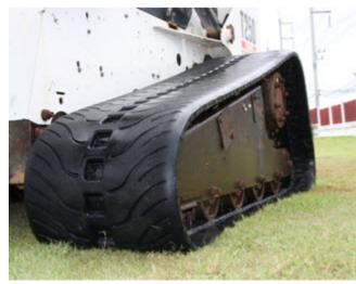
While many construction pros drool over rubber tracks with aggressive traction for their advantages in a variety of construction applications, landscapers frown at the site of aggressive traction pattern on rubber tracks.
