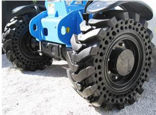
Stability is one of those factors that highly improve the efficiency of telehandlers on the jobsite. Specifically, the elimination of equipment bouncing, which sometime occurs with pneumatic tires, can greatly improve the ability of the operator to safely use the machine. This is even more important when the high reach telescopic forklift will be used to carry construction materials around the site with an extended boom.
