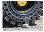
backhoes don't use an axle mounted suspension, they are vulnerable to vibrations from the ground, which makes Nu-Air's superior shock-absorption an even more welcoming feature. Add to this the zero chance to ever get flats, and you got an undisputed winner."
