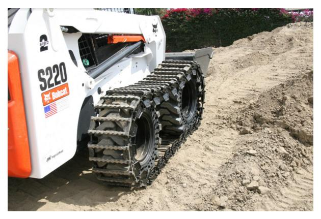
One of the best upgrades that you can get for a skid steer loader with tires is <u>over-the-tire skid steer tracks</u>. From expanding the capabilities of your machine to increasing its revenue potential, there are numerous advantages that these versatile tracks offer. To learn about some of the most impactful benefits of over-the-tire skid steer tracks, continue reading.
