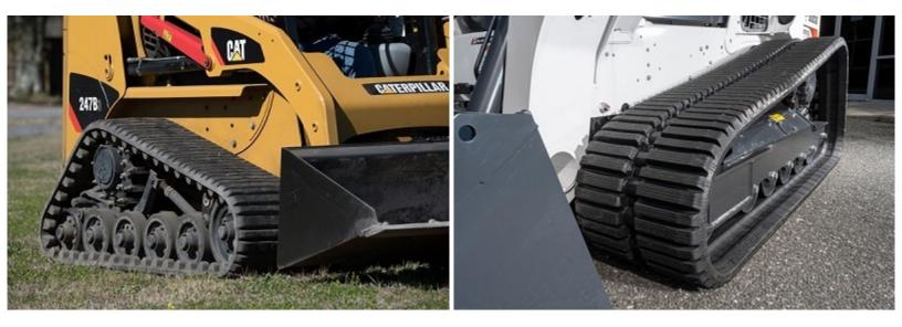
CTL and MTL (ASV type) machines are both popular track loader options. There are many different factors to consider when determining which of these similar machines is best for your application. One such consideration is whether Compact Track Loader or Multi Terrain Loader **<u>rubber tracks</u>** are more advantageous for your purposes. This guide on the **difference between CTL vs MTL rubber tracks** will help guide your decision.
