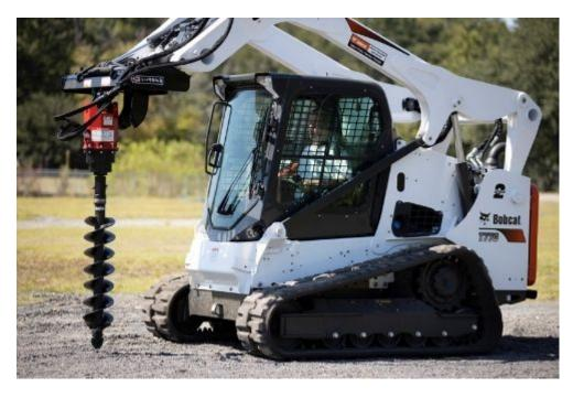
Skid steer owners have the opportunity to widely expand the capabilities of their machine by fitting it with a vast range of attachments. One of the most useful skid steer attachments on the market is an auger. A <u>skid steer auger</u> is an attachment designed to pierce the ground and drill straight down. In doing so, this attachment proves useful in a wide range of applications. Discover some of the many uses of skid steer augers.
