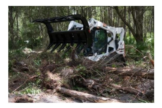
Skid steers are versatile pieces of machinery. Useful for an array of applications, skid steers are especially helpful when tackling landscaping and construction projects. Their relatively lightweight construction and easy maneuverability makes them agile and particularly beneficial for spreading dirt, digging, mowing, and land clearing.
