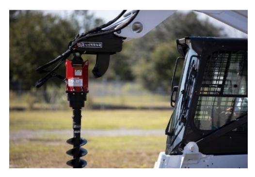
Skid steer and mini excavator augers are among the most popular and important aftermarket products for compact equipment. Whether it be the construction or landscaping industry, these devices are incredibly useful for boring into the toughest of ground conditions. As such, having one of these products is a must if you're looking to use your compact equipment for more projects than material transportation.
